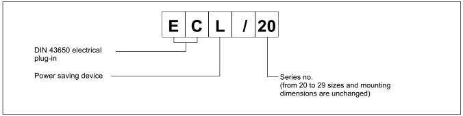
The ECL connector is a digital amplifier controlling open loop on-off valves directly from PLC.
